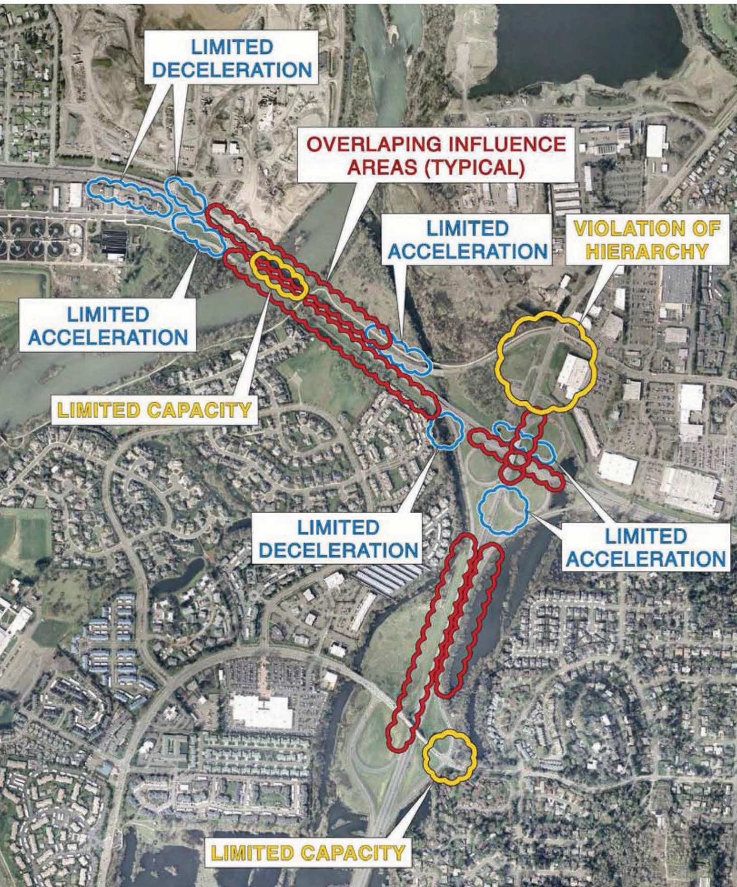
FIGURE 4 Deficiencies on Beltline Beltline Highway: Coburg Road to River Road Facility Plan CH2MHILL
